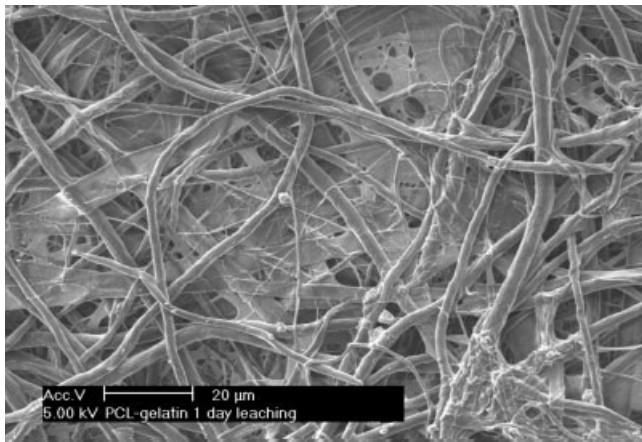
Figure 2 SEM image of G50 dissolved in DI water for 1 day at 37°C showing partial and nonuniform dissolution. Note that cell-like morphologies are produced by partial dissolution even in the absence of cells.
